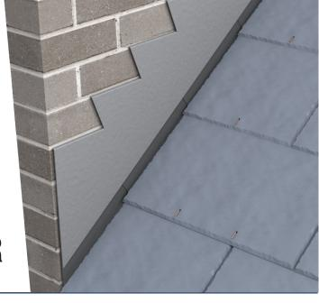
Kytun™ Aluminium soakers are a lightweight and durable alternative to lead. They are used when forming a pitched roof against an existing wall.
