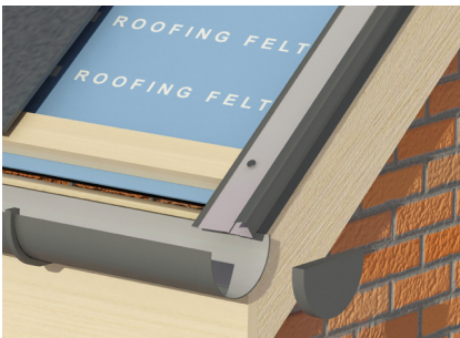
Fig.1. Nail each length of trim to batten.
