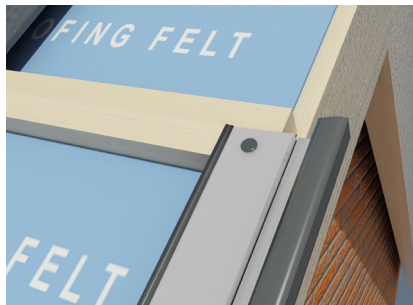
Fig.2. Join at the centre of the batten.
