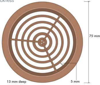
For 10mm continuous ventilation install at 200mm centres, for 25mm continuous install at 80mm centres.
