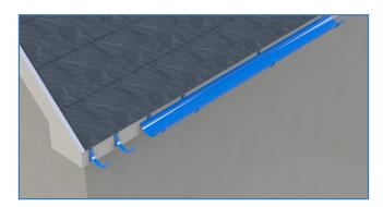
4. Once all brackets are secured, starting from left to right, hook and snap gutter into position. Secure system in accordance with the jointing process (see overleaf).
