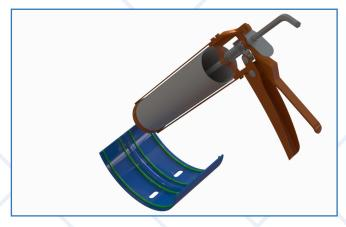
3. Apply 2 no. generous 10mm beads of sealant to either side of drilled holes and around bolt hole in the lengths being joined. Re-position the jointer ensuring the holes are aligned. Insert M6 x 16 stainless fixing bolts from the underside of the gutter. Do not over tighten.
