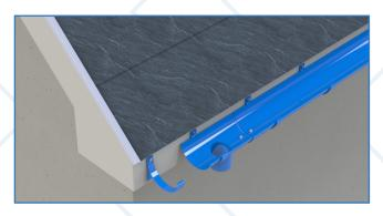
Position outlets using a plumb line to gullies at ground level. Each outlet should have 1no bracket directly supporting it.
