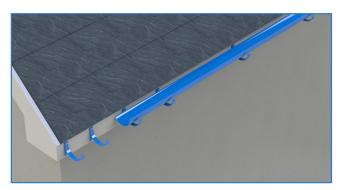
3. Using the string line, set out brackets at 750mm to 900mm centres at a 1:600 to 1:1350 (max) fall. Alternatively, set the line as nominally level. Allow for 4no brackets per 3.0m gutter length, 1no per angle and 1no per outlet.
