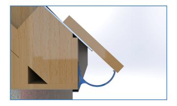
1. Starting at a corner or end, place a spirit level or straight edge on top of the tiles or slates. Offer up the gutter fascia bracket to the underside of the straight edge and mark the screw hole.
