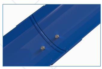
4. Remove any surplus sealant from faces of gutter. Using the sealant gun, ensure all areas around the jointer, length and fixing nuts are sealed with the bonding sealant. Gutter bolts may be touched up using touch up paint provided.
