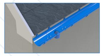
6. Continue to install gutters, angles and outlets with internal / external jointers as required.
