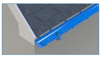
7. End cap to be placed in position, drilled and fixed as per the jointing process.
