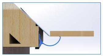
1. Starting at a corner or end, position a spirit level against the lowest edge of a tile or slate and offer up the gutter fascia bracket. Check fascia board alignment and shim where necessary. (See Page 3 for alternative gutter position.)
